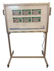
It incorporates real OEM EV components including cables and connectors as well as a Service Disconnect Plug. These can be disconnected and voltage measurements can be performed using the test points provided. The 12V Battery can also be disconnected to allow the user to perform EV disabling exercises.
