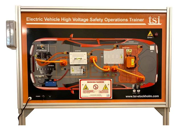
This mobile training stand has been specifically design to teach the principles of safe working on Electric Vehicles.
